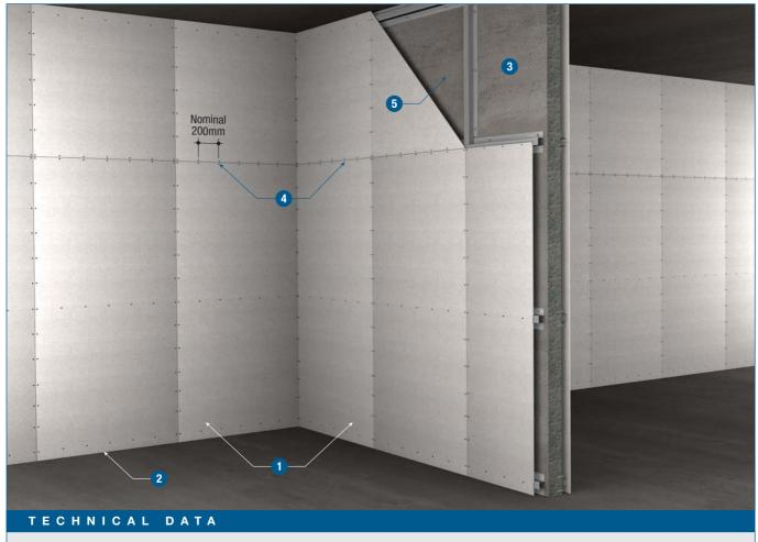
For increasing the fire resistance from 60 to 120 minutes 1 layer of PROMATECT®-H board 9mm thick, fixed with steel hats to each side of concrete or brick wall. See page 2 for the required thicknesses of wall and gypsum plaster where applicable.
